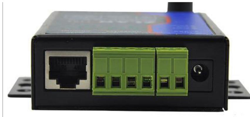
**Figure 4 Front Interfaces of ITT-SR4780**
