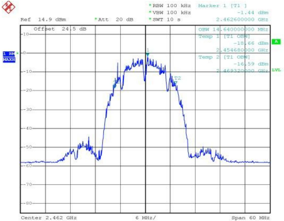
Figure 11 ITT-SR4780 Bandwidth Test Curve
