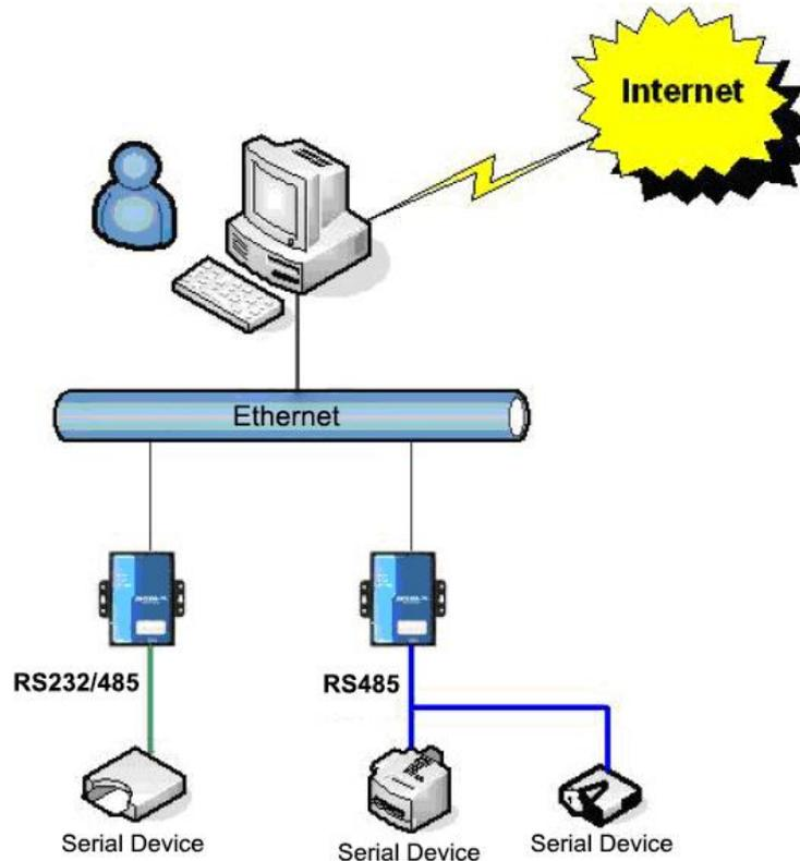
Figure 2 ITT-SR4780 Network Structure
