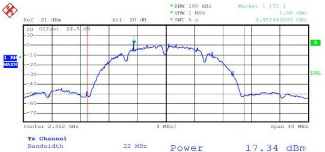
Figure 12 ITT-SR4780 Power Test Curve
