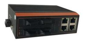
The ITT-4FE4FX-I-DC provides 4 electrical Fast Ethernet ports and 4 optical Fast Ethernet port. All models are with IP40 protection class and meet EMC industrial level 4 requirements. It provides 12-36 VDC wide voltage range power inputs, DIN rail mounting, wide operating temperature range of -40 to the +85°C. In addition to its compact size for space-saving installation, each product has passed a 100% burn-in test in 85°C to ensure its quality.
