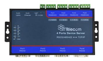
ports, realize 4 ports simultaneous full-duplex working by connecting to ITT-SC4763 via a cable. It's the ideal choice of multiserial ports networking.
