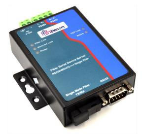
ITT-SRLAN9153 fiber serial device server is an industrial serial port to fiber converting device developed by Ittelecom. The device can realize transparent transmission between 1 channel RS232/RS485/RS422 data and fiber.
