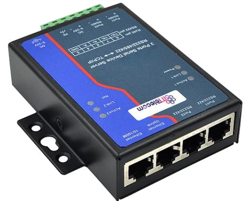
ITT-SR4211 serial device server is a 2 ports protocol converter between RS232/485/422 and TCP/IP developed by ITTELECOM. ITT-SR4211 support 2 RS232 ports, 2 RS422/485 ports, can realize 2 serial ports simultaneous full-duplex working through connecting to ITT-SR4211 via a cable. The RS485 interface is green terminal interface, the RS232/RS485 are RJ45 Ethernet port connection interface.
