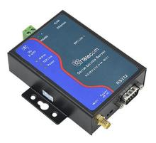
High performance industrial serial port to WIFI serial device server, support RS232/485 to WIFI. 9~24V power supply, support Modbus TCP to RTU. Support (IEEE802.11g/b/n) protocol. Support virtual serial port.
