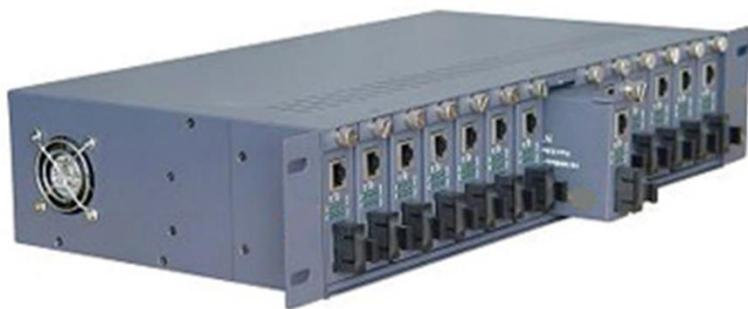
It is acceptable for the most 14 sets of 10M/100M, or 10/100/1000M Stand alone Media Converters within a rack-mountable chassis which is supplied with unified power. Installing at the center of network, the Rack not only reduce the links, simplify the structure, but also ease for management and maintenance.
