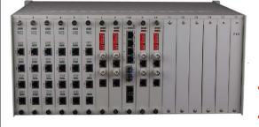
256 POTS (FXO/FXS) over Fiber multiplexer is a kind of point-to-point fiber transmission device. ITTELECOM designed 1~256POTS (FXO/FXS), it is a multi-service fiber multiplexer which can realize 256channel voice and 4\*Fast/ Gigabit ethernet over fiber transmission. The fiber multiplexer is rack mount device which have 16slots for 16voice card or E1 card. The device support SNMP and console management. P/N : <u>ITT-MU4101</u>
