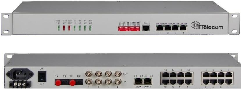
This device provides 16Channel telephone, 1-4Channel E1 interface, 4Channel 10M/100M Ethernet interface (Wire Speed 100M) and 4 expansion interface. 4Channel Ethernet interface is switch interface, can support VLAN. 4 expansion interface can be used as the transmission channel of RS232/RS485/RS422 asynchronous data, voice signal, 2/4 line E&M audio signal, switch signal, Ethernet signal (Bandwidth 2M). It is very flexible.
