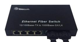
The ITT-MC4370 is a POE switch designed for network monitoring. It has four 10/100/1000Mbps Ethernet ports and two 1.25Gbps fiber ports. It is designed with imported Marvell chip, lower power consumption and high stability. It extends the transmission distance of a network from 100m to120km via copper cables. It can extend the transmission distance, and also have many other advantages such as isolation protection, good data security, working stability and easy maintenance.
