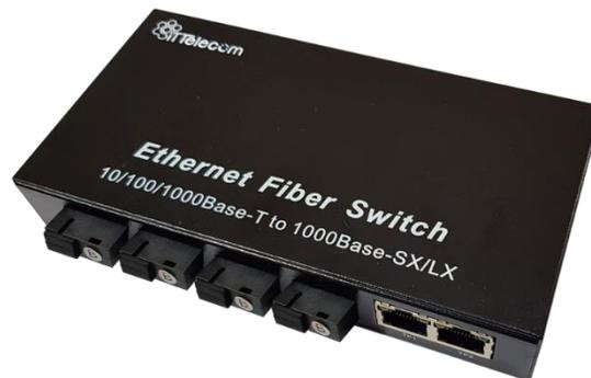
The ITT-MC4F2E is a 10/100Mbps adaptive fast Ethernet fiber switch designed for network monitoring. It has two 10/100Mbps Ethernet ports and four 155Mbps fiber ports. It extends the transmission distance of a network from 100m to 120km via copper cables. There are also many other advantages such as isolation protection, good data security, working stability and easy maintenance.
