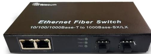
The ITT-MC1891 is a 10/100/1000Mbps adaptive gigabit Ethernet Fiber Switch. It has two 10/100/1000Mbps Ethernet ports and two 1.25Gbps fiber ports. It extends the transmission distance of a network from 100m to 120km via copper cables. There are also many other advantages such as isolation protection, good data security, working stability and easy maintenance.
