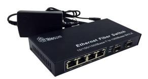
The ITT-MCP-4GE2SFP is a POE switch designed for network monitoring. four 10/100/1000Mbps Ethernet ports and two 1.25Gbps fiber ports. It is with imported Marvell chip to designed achieve lower power consumption and high stability. It extends the transmission from 100m distance of а network to120km via copper cables. There are also many other advantages such as isolation protection, good data security, working stability and easy maintenance.
