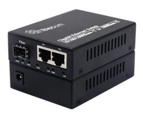
The ITT-MC-2GE1SFP is a 10/100/1000Mbps adaptive gigabit Ethernet Fiber Switch. It has two 10/100/1000Mbps Ethernet port and one 1.25Gbps fiber port. extends transmission distance from 100m to 120km via copper cables. There are also many other advantages such as isolation protection, good data security, working stability and easy maintenance.
