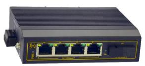
The ITT-ISW-4G1S provides 4\*electrical Fast Ethernet ports and 1\*optical Fast Ethernet port. All models are with IP40 protection class and meet EMC industrial level 4 requirements. It provides 12-36 VDC wide voltage range power inputs, DIN rail mounting, wide operating temperature range of -40 to the +85°C. In addition to its compact size for space-saving installation, each product has passed a 100% burn-in test in 85°C to ensure its quality.
