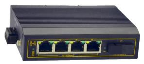
The ITT-SW3911 provides 4\*electrical Fast Ethernet ports and 1\*optical Fast Ethernet port. All models are with IP40 protection class and meet EMC industrial level 4 requirements. It provides 12-36 VDC wide voltage range power inputs, DIN rail mounting, wide operating temperature range of -40 to the +85°C. In addition to its compact size for space-saving installation, each product has passed a 100% burn-in test in 85°C to ensure its quality.
