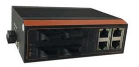
The ITT-ISW-4G4S provides 4 electrical Fast Ethernet ports and 4 optical Fast Ethernet port. All models are with IP40 protection class and meet EMC industrial level 4 requirements. It provides 12-36 VDC wide voltage range power inputs, DIN rail mounting, wide operating temperature range of -40 to the +85°C. In addition to its compact size for space-saving installation, each product has passed a 100% burn-in test in 85°C to ensure its quality.
