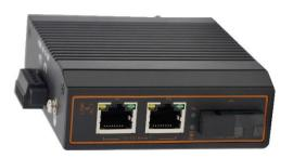
The ITT-SW3905 provides 2\*electrical Fast Ethernet ports and 1\*optical Fast Ethernet port. All models are with IP40 protection class and meet EMC industrial level 4 requirements. It provides 12-36 VDC wide voltage range power inputs, DIN rail mounting, wide operating temperature range of -40 to the +85°C. In addition to its compact size for space-saving installation, each product has passed a 100% burn-in test in 85°C to ensure its quality.
