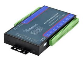
ITT-SC4768: Compared with 6842, 6844 adds WiFi interface, it can save the wiring trouble. Meanwhile it has Ethernet interface. WiFi can be neither as AP nor as SAT style to connect router.
