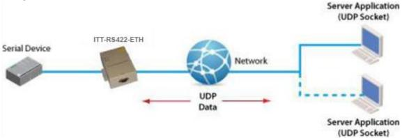
UDP based applications, convert serial equipment data for transport across UDP packets either on a point to point basis or shared across multiple devices.
