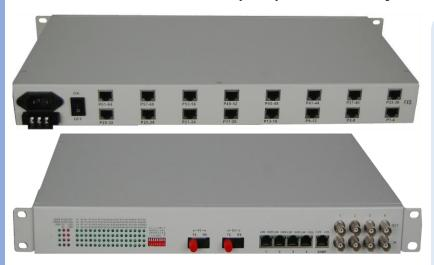
This product is a 19 inch 1 U rack installation, 64channel voice, 4channel E1 interface, 4\*10M/100M Ethernet interface. Four Ethernet interface for the exchange, can support VLAN. Support SNMP or Console Management. Fiber 1+1 back up for option. The application is very flexible. Have perfect alarm function, the machine work stable and reliable, low power consumption, high integration, small volume.
