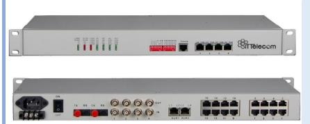
provides This device 16Channel telephone.1-4Channel E1 interface, 4Channel 10M/100M Ethernet interface (Wire Speed 100M) and 4 expansion interface. 4Channel Ethernet interface is switch interface, can support VLAN. 4 expansion interface can be used as the channel of RS232/RS485/RS422 transmission asynchronous data, voice signal, 2/4 line E&M audio signal, switch signal, Ethernet signal (Bandwidth 2M). It is very flexible.
