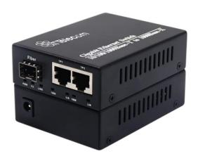
The ITT-MC4469 is a 10/100/1000Mbps adaptive gigabit Ethernet Fiber Switch. It has two 10/100/1000Mbps Ethernet port and one 1.25Gbps fiber port. It extends the transmission distance from 100m to 120km via copper cables. There are also many other advantages such as isolation protection, good data security, working stability and easy maintenance.
