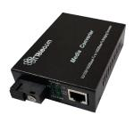
The ITT-MC2159 is a 10/100Mbps adaptive media converter. It can transfer 100Base-TX of electrical signals to 100Base-FX of optical signals. It can extend the transmission distance from 100m to 120km via copper cables. There are also many other advantages such as isolation protection, good data security, working stability and easy maintenance.
