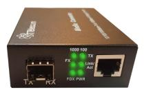
The ITT-MCSFP1G1E is a 10/100/1000Mbps adaptive gigabit Ethernet Fiber Switch. It has one 10/100/1000Mbps Ethernet port and one 1.25Gbps fiber port. It extends the transmission distance from 100m to 120km via copper cables. There are also many other advantages such as isolation protection, good data security, working stability and easy maintenance.
