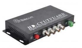
The converter can simultaneously transmit 1-16 channels HD-CVI/TVI/AHD over one multitude or single-mode optical fiber. LED indicates instantly monitoring system status. Devices are available for either standalone or rack-mount installation, which is suitable for different working environment. Compatible with AHD-H, AHD-M, AHD-L. It is without loss and non-compression real time transmission.
