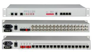
This device provides 1-16\*E1 interface, 1-4\*10M/100M Ethernet interface (Wire Speed 100M) and 2 expansion interface. 4\* Ethernet interface is switch interface, can support VLAN. 2 expansion interface can be used as the transmission channel of RS232/RS485/RS422 asynchronous data. It is very flexible. It has alarm function. The work is reliable, stable, and low power consumption, high integration, small size.
