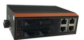
The ITT-SW3912 provides 4 electrical Fast Ethernet ports and 4 optical Fast Ethernet port. All models are with IP40 protection class and meet EMC industrial level 4 requirements. It provides 12-36 VDC wide voltage range power inputs, DIN rail mounting, wide operating temperature range of -40 to the +85°C. In addition to its compact size for space-saving installation, each product has passed a 100% burn-in test in 85°C to ensure its quality. All of these features make the product ideal for
